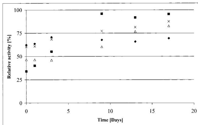
FIG. 3. Effect of HM508 degradation on enzyme inhibition. Enzyme activities are expressed relative to the activity in the samples without inhibitor; ChiB wild type (triangles), ChiB-M212A (squares), ChiB-D142N (diamonds), and ChiB-W220A (crosses).
