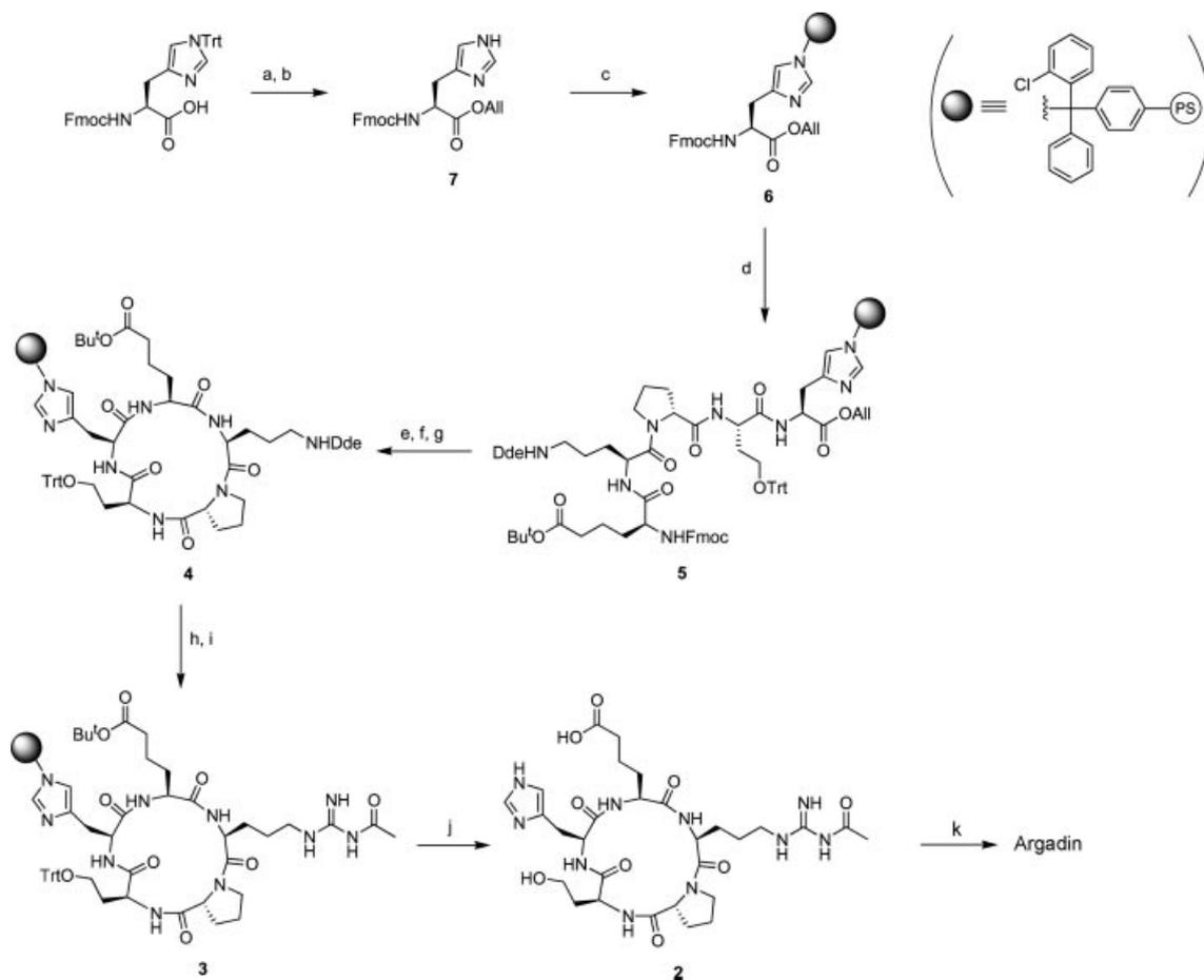
Scheme 2. a) allyl alcohol, DCC, DCM, 65%; b) TFA/DCM/TIPS (10:9:1), 95%; c) 2-chlorotrityl chloride polystyrene resin, DIPEA, DCM; d) Fmoc SPPS; e) Pd(Ph<sub>3</sub>P)<sub>4</sub>, PhSiH<sub>3</sub>, DCM; f) piperidine/DMF (1:4); g) PyBOP, DIPEA, DCM; h) H<sub>2</sub>NNH<sub>2</sub>/DMF (1:49); i) acetyl methylthiourea hydroiodide, DIPEA, DMF; j) TFA/DCM/TIPS (10:9:1), 10% from 6; k) IBX, DMSO, 71%.
